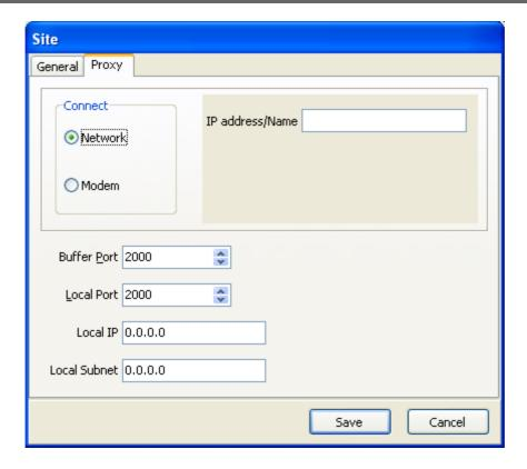
The proxy allows a bridge between an unencrypted TCP/IP local connection and a remote, encrypted NetBuffer or ModemBuffer. The remote buffer should be configured for Serial->TCP2, TCP1->TCP2 (for the NetBuffer), or r210="T" (ModemBuffer).
